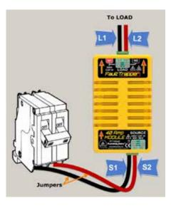
1. Remove the two hot wires from the breakers for the load being tested and attach them to the Load side of the Fault Trapper 40A In-Line Adapter Module with the black in Load Terminal "L1" and the red wire in Load Terminal "L2" using the Plug-in Terminal Block Connector.
